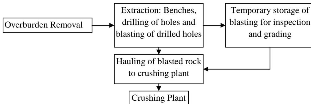
**Figure 1:** Process Flow Diagrams for Granite Quarrying Operations
